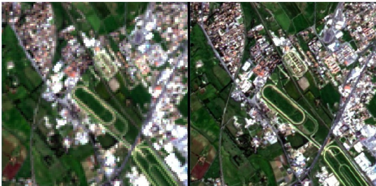
Fig. 14: Example of pan-sharpening of a Landsat 8 image. Left, original multispectral bands (30m); right, pan-sharpened bands (15m)
